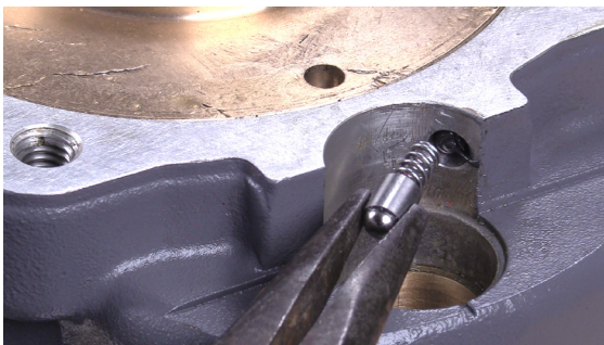
Install Reverse Lock Plunger and Spring Assembly.
