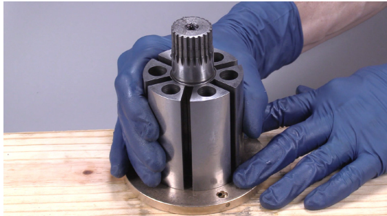
Remove Rotor from Rear End Plate.
