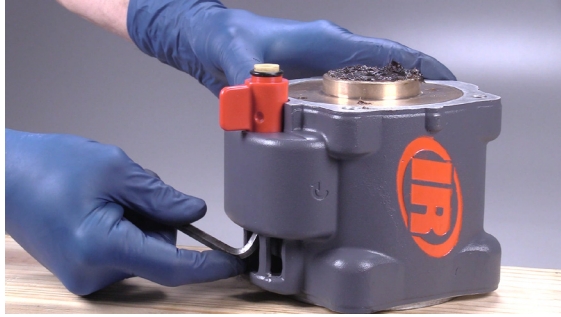
From the Exhaust Outlet use the short end of the 1/4" Hex wrench to press the Reverse Valve upwards.
