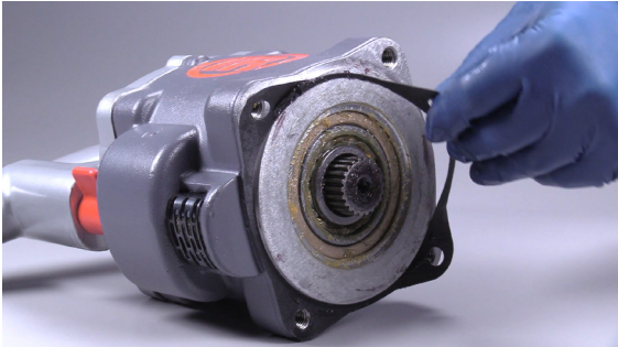
Remove Hammer Case Gasket.
