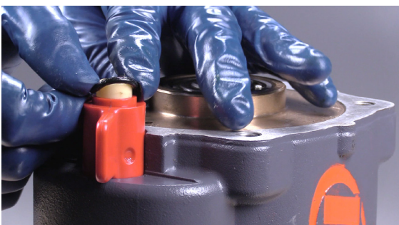
Install Reverse Valve Seal.
