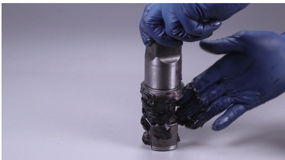
Fill the lugs on the Anvil with #170 IR grease.
