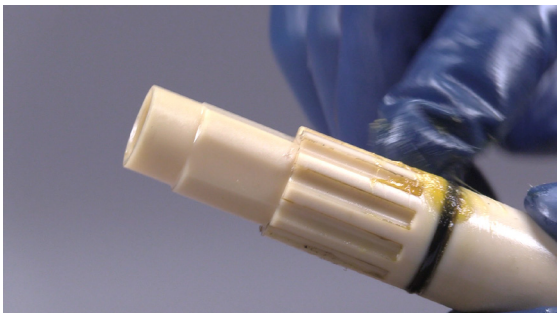
Lubricate Reverse Valve o-ring with o-ring lubricant.
