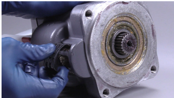
Pinch the Exhaust Guard upward to dislodge and remove it.
