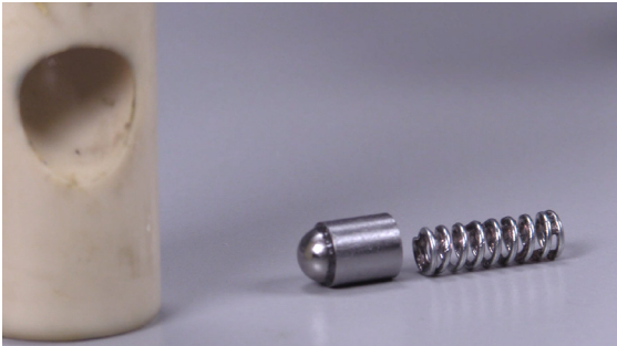
Reverse Lock Plunger and Spring Assembly
