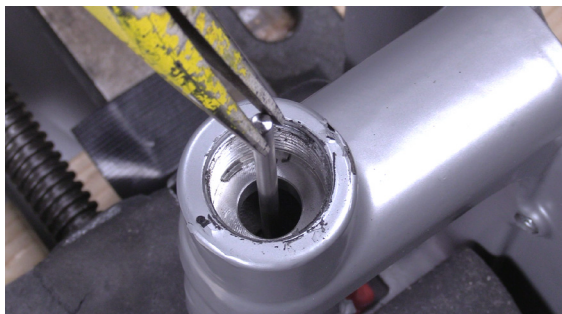
Remove Throttle Valve Plunger.
