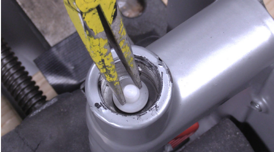
Remove Throttle Valve Seal.
