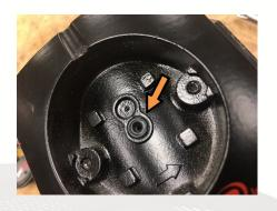
Be especially careful not to lose the small O-Rings that seal the Gauge and Block to the Regulator Body.
