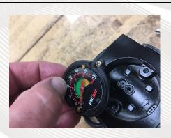
Install the Gauge, where the Block had been. Secure using the two Phillips-head Screws. Then re-install the Gauge Cover.
