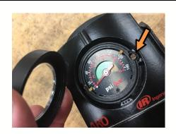
To relocate the Gauge, remove the front Gauge Cover Ring.
