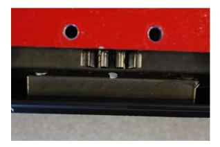
10) Seat the pinion gears with the rack gears on the drive board. If the gears are aligned properly, the drive board will seat with little to no movement of the gears. Install both guide plates.
