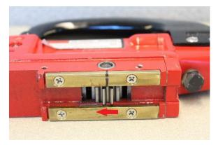
3) Locate the left-most gear tooth that is not inside the body of the tool.
