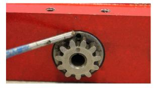
8) Mark the center tooth of the reverse valve rack gear (center gear on drive board)
