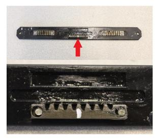
9) Ensure that all gear teeth are still aligned properly with their marks, and align the marked gear tooth with the timing dot on the reverse valve pinion.
