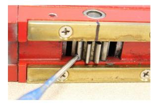
4) Rotate the gear counterclockwise, until this tooth lines up with the mark made on the wear plate. Rotate the gear counterclockwise an additional 3 teeth, and stop.
