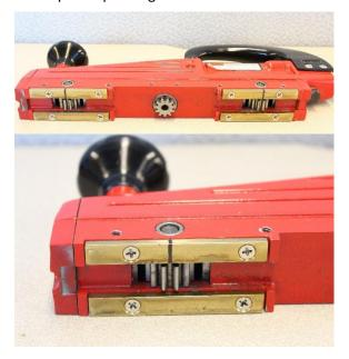
2) Rotate both piston pinion gears towards the front of the tool (clockwise when viewed from above) until they stop.
