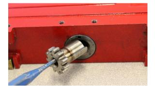
7) Align the timing dots on the pinion and the bushing.
