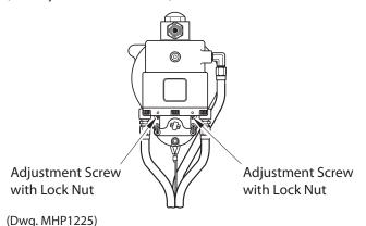
For maximum performance and control, adjust the bleed screws (19) or (336 [old style]) as follows:
